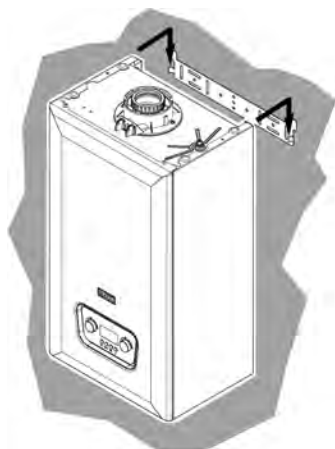
Fig.30 Mounting the boiler
