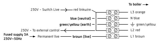
Connect external control using L2 & L3
