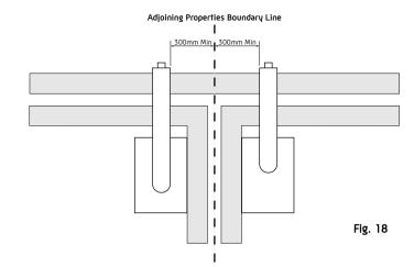
NOTE: The minimum distance from a flue terminal to a boundary line is 300mm.
