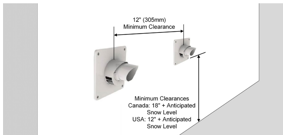
Figure 11a: Horizontal Concentric Termination - Two Kits
