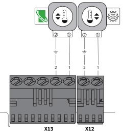
Frost thermostat and OpenTherm thermostat connection
