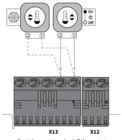
Frost thermostat and on/off thermostat parallel connection
