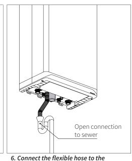
Connect the flexible hose to the sewer via an open connection.
