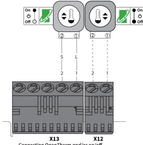
Connecting OpenTherm and/or on/off room thermostats
