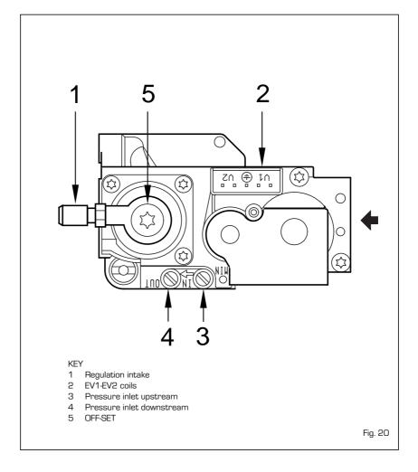
To increase working pressure, turn the trimmer clockwise; to reduce pressure, turn the trimmer counterclockwise.
