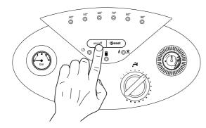
Should the boiler fail to ignite a second time, check that the external gas cock is open. If the problem persists, contact an Authorised Service Centre.
