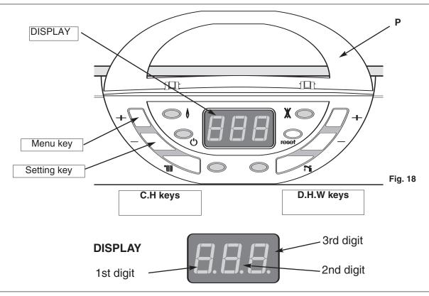
To gain access to the setting menus press both the — and + keys on the D.H.W. side for 5 seconds. (Fig. 18). Menu 1 is displayed.
