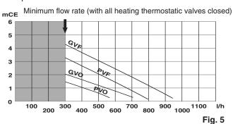
Pump head chart available at the outlet of the boiler Central heating initial pressure when cold (in bar)
