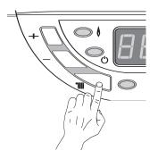
Press on key 32 \*\*\* , the green indicator 33 will light and the display will show the Heating flow temperature.
