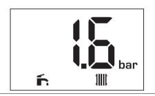
The filling pressure in the heating installation and the operating mode are shown in the display's basic display.
