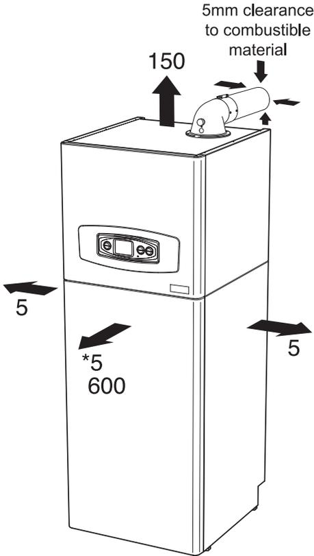
\*A removable compartment door can be placed a minimum 5mm in front of the appliance. A clearance of 600mm is required from a fixed surface.
