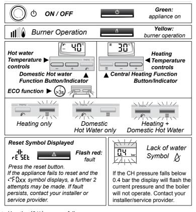
If the central heating (C.H.) pressure falls below 0.4 bar the display will flash the current pressure and below 0.3 bar the boiler will not operate, refer to fault finding section.
