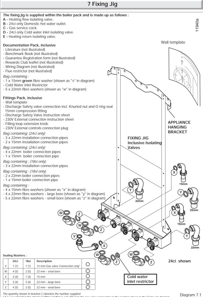
\* It is essential that this green sealing washer is only fitted to the gas valve connection in the position shown in the Fixing Jig diagram
