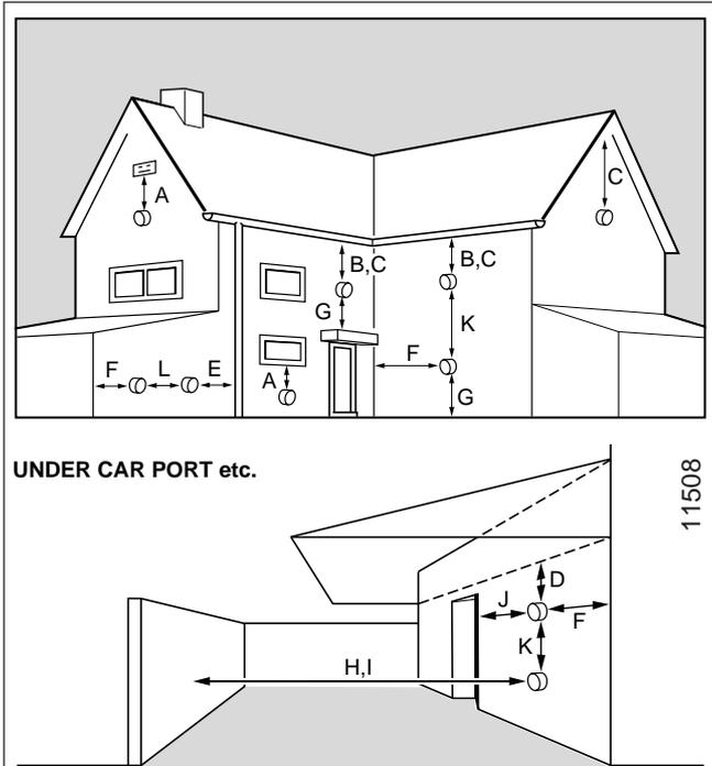
**MINIMUM SITING DIMENSIONS FOR FANNED FLUE TERMINALS POSITION** **MM**
