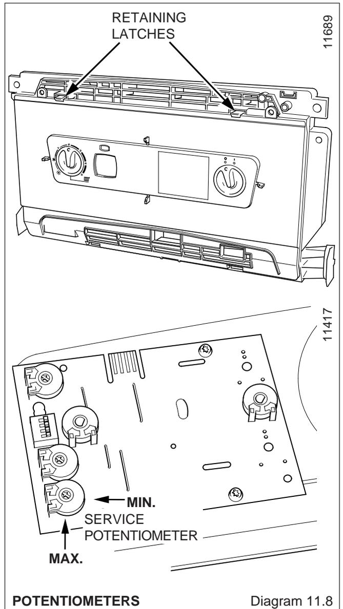
Adjust the maximum rate CO<sub>2</sub> with the throttle to 8.8%. (Rotate anti-clockwise to increase).
