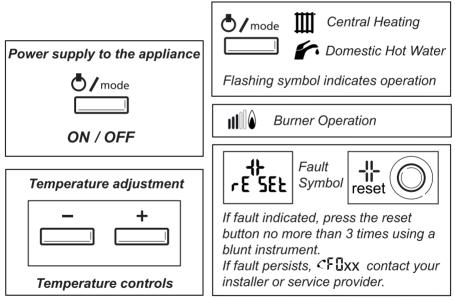
This Quick reference guide assumes that the appliance have been installed and commissioned by a competent person. If the central heating (C.H.) pressure falls below 0.5bar the display will flash the current pressure and the boiler will not operate, refer to fault finding section. We designed this Quick reference guide so that you can start using your appliance right away.
