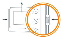
Remove the front panel of the thermostat by squeezing the buttons on both sides and sliding it up and off the backplate.
