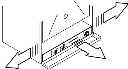
When completely pulled out, the panel can rotate 45° downwards to facilitate access to the internal parts.
