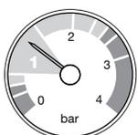
**Central Heating System Pressure** - The normal operating water pressure is shown when the needle is between 1 and 2.5 bar. If the pressure exceeds 3 bar the safety pressure valve will operate and a fault is indicated. Contact your Installer.
