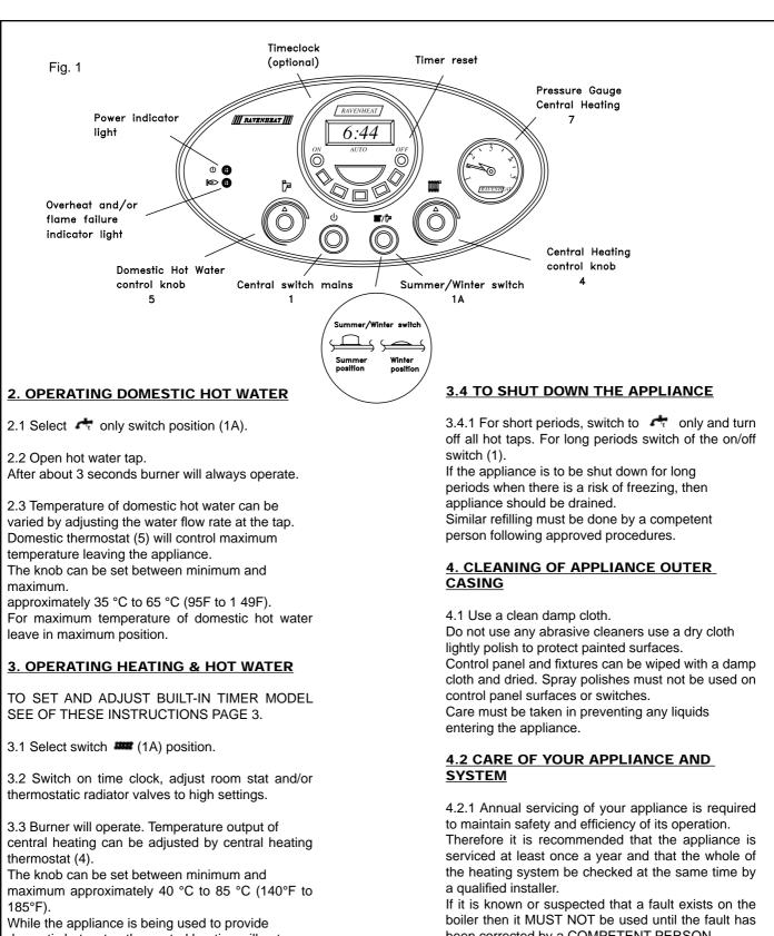
domestic hot water, the central heating will not operate. When hot water is no longer required the appliance
