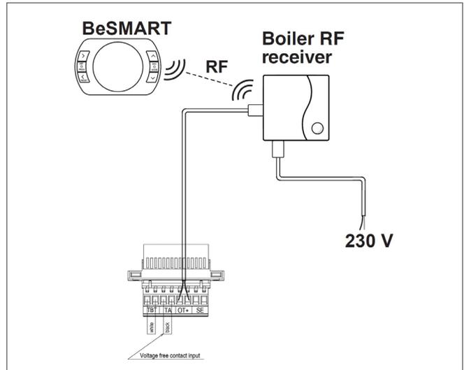
**8.11 TYPICAL CONNECTION FROM REMOTE ROOM THERMOSTAT AND CLOCK – CONNECTED TO THE 8-POLES CONNECTOR**
