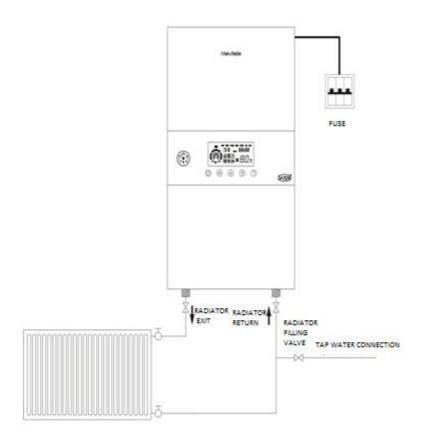
After hydraulic connections are made, filling the heating system is necessary. For the model of UKDAX –xxET Tand UKDAX –xxEDM this process is made with filling valve connected to heating system. For this, connection with valve must be made from cold water installation to heating system. This valve must placed near place to device because of it will be used for filling the heating system and must be position as it can be seen pressure indicator when the
