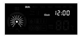
Keep press \_ ② 2 seconds. If setting heating mode of the device was radiator modebefore it is OFF, after pump is operated about 1 min, device start to radiator heat and \_ ⑥ n is seen inside display. If the setting of the device was water heating before it is OFF, it stays in standby mode for hot water using. Warning beep is heard after every pressing knob process. For long time pressing knobs (for example 2-3 seconds), before hearing warning beep, it does not mean pressing knob.
