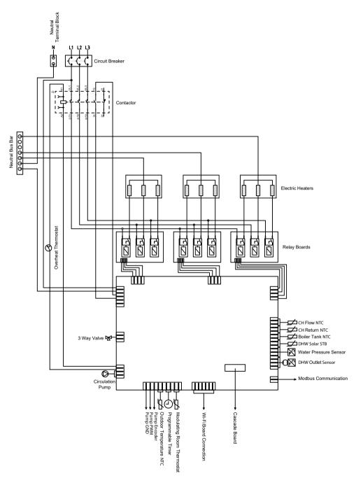
Figure 3. Arceus 18-24 kW Wiring Diagram
