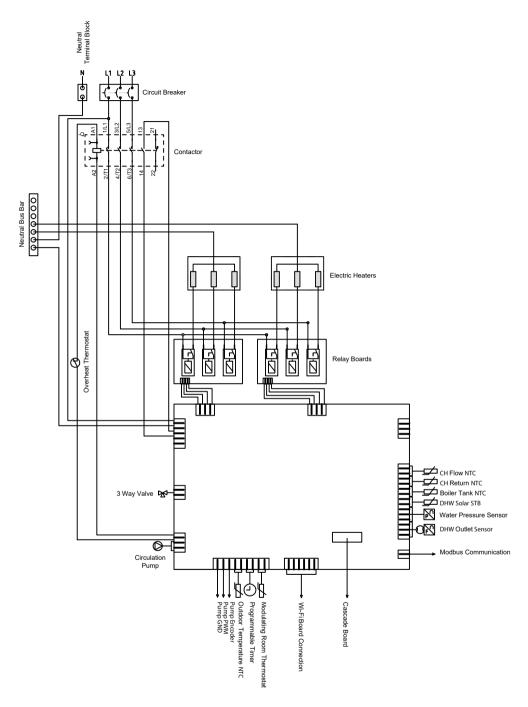
Figure 2. Arceus 12-15 kW Wiring Diagram
