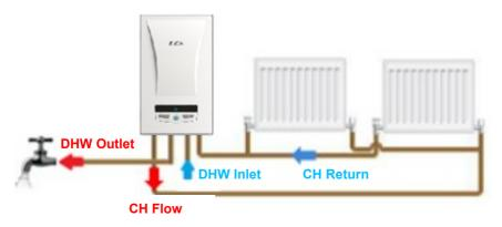
Figurel 7. Monothermic Device Installation Scheme
