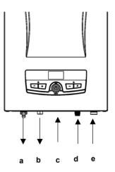
Figure 14. ST boiler water connections
