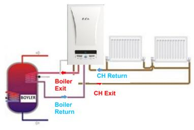
Figure 9. ST Device Installation Scheme
