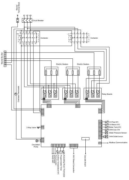
Figure 4. Arceus 27 kW Wiring Diagram
