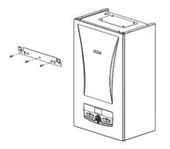
Figure 11. Bracket Assembly
