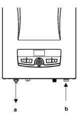
Figure 13. CH boiler water connections
