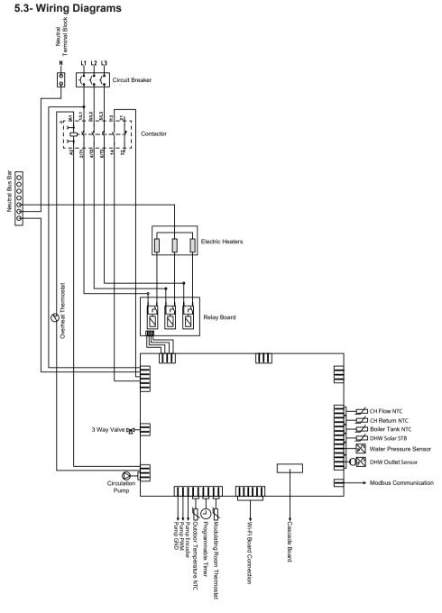
Figure 1. Arceus 6-9 kW Wiring Diagram
