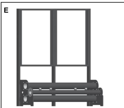
A Position the pipe work header in the required location. When using several pipe work headers: couple the pipe work headers using the supplied gaskets, M12 (DN65) or M16 (DN100) bolts, spring washers and nuts. Align the pipe work header(s) horizontally using the adjustable feet.
