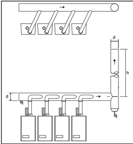
Diameter and venting lengths of the flue gas outlet/air supply:
