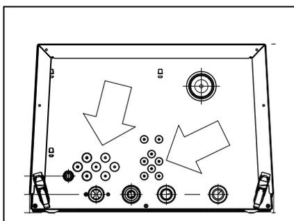
PG glands for cable duct already assembled in the factory. For a few connections, some PG glands are supplied separately.
