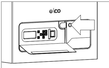
Open the flap by pushing right next to the flap on the round button to reach the display and keyboard.
