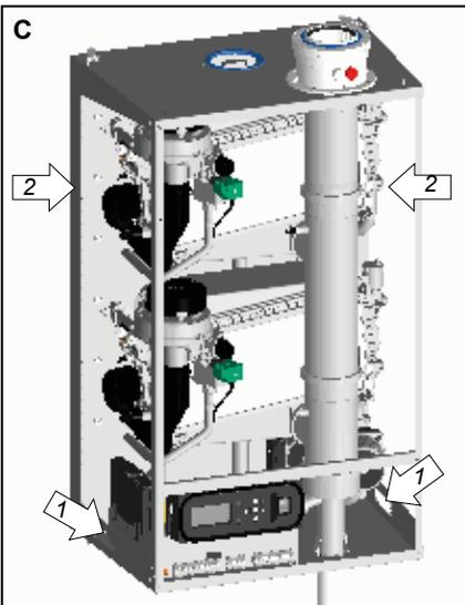
C. Hang the boilers on the suspension brackets. **Lift the boiler only by the special grips on the bottom panel (1) and support the boiler by its rear panel (2).**
