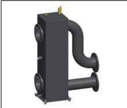
The low loss headers comes standard with adjustable feet, automatic air vent, drain valve, pocket for temperature sensor T10, M12 or M16x55 bolts, spring washers and nuts. The low loss header can be positioned on either the left or right hand side of the pipe work headers.
