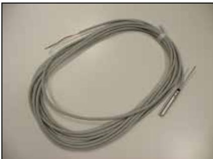
Every system with 1 or more THISION L ECO-boilers must be provided with a flow temperature sensor T10 and must be connected on the master boiler (address 01) to terminal 3, position 5 and 6. The flow sensor must be placed in the pocket of the low loss header.
