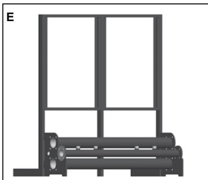
A. Position the pipe work header in the required location. When using several pipe work headers: couple the pipe work headers with the supplied gaskets, M12 (DN65) or M16 (DN100) bolts, spring washers and nuts. Align the pipe work header(s) horizontally using the adjustable feet.
