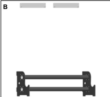
B. Determine the position of the suspension brackets based on figure B1. The boilers can be fitted on the wall using the supplied suspension brackets and mounting material (minimum of 3 screws for each boiler). The wall has to be flat and strong enough to carry the weight of all boilers including their water contents.
