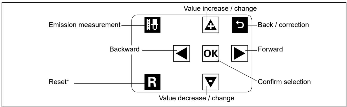
The keyboard consists of a logical button allocation for menu control, confirmation, and correction and emission measurement.
