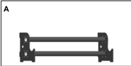
A. Position the pipe work header against the wall. When using several pipe work headers: couple the pipe work headers and supplied gaskets, M12 (DN65) or M16 (DN100) bolts, spring washers and nuts. Align the pipe work header(s) horizontally using the adjustable feet.
