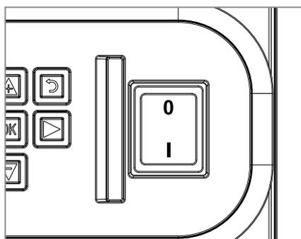
The main switch is located on the right hand side of the keyboard. This switch controls the 230V power supply (L and N).
