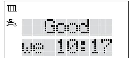
Good indicates that the boiler operates normally (burner on or off) wo 10:17 indicates the actual day and time.
