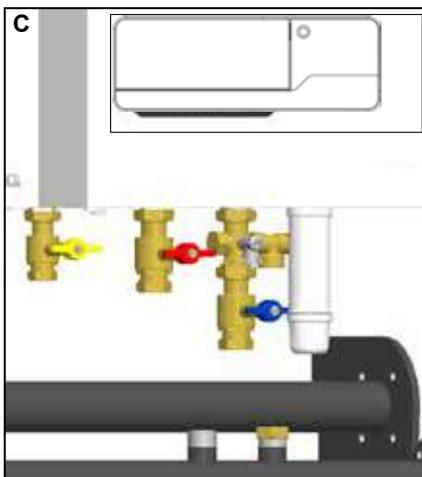
**Polluted test water may be released when removing the plastic caps on the boiler flow and return.**
