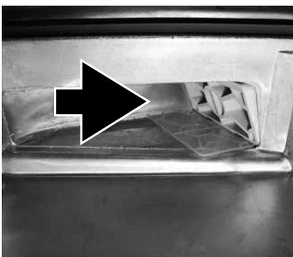
If the cover/air box is heavily polluted with dust, it is likely that the fan impeller is also polluted. To clean the fan, it has to be removed from the upper tray and the venturi. Clean the impeller with a soft brush and a vacuum cleaner. Replace the gasket and take care that the new gasket is installed properly when reassembling the fan parts.
