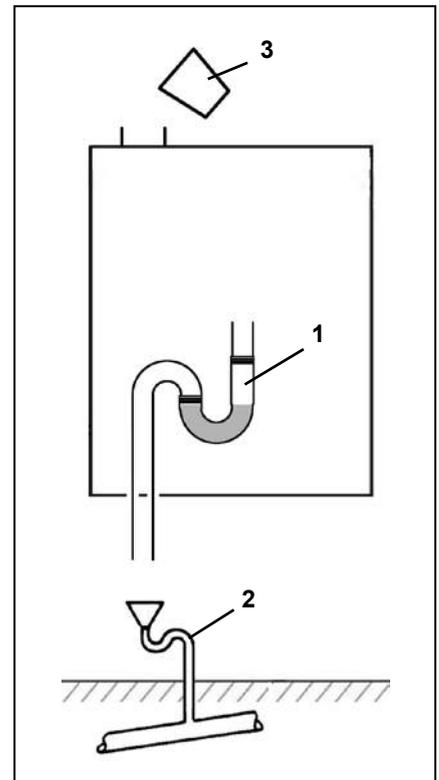
All ELCO wall hung gas fired condensing boilers contain a siphonic condensate trap to collect and release condensate.
