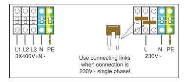
The terminal connection block is located mid-way up at the front left hand side of the boiler and is accessed after removing the boiler front panel. The supply cable should be routed to this point through the cable entry point on the left hand bottom of the boiler.
