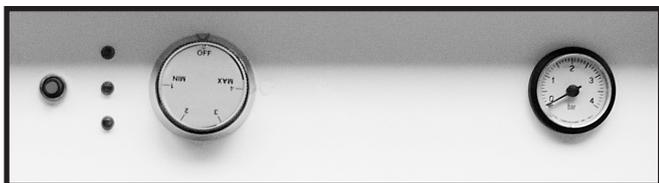
This is the control knob which can regulate, within the band 50 - 80°C, the temperature of the boiler water, known as primary water, which is the water which runs through your radiators and heating system.
