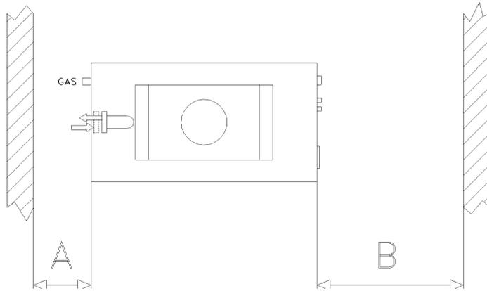
Allow minimum of 5 mm at sides of boiler for assembly
