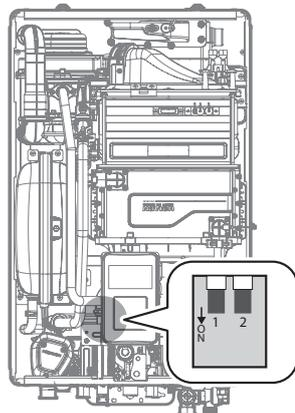
Figure 6. Set the DIP switches
