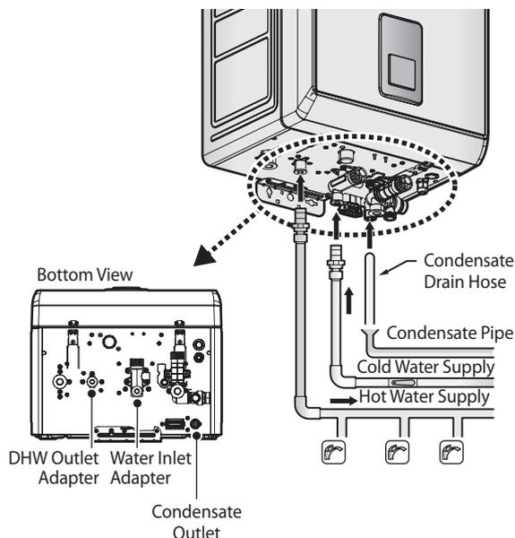
**Note** If the cold water supply pipe is fitted with water meter, check valves or loose jumper stop cock, then a DHW expansion vessel must be fitted.
