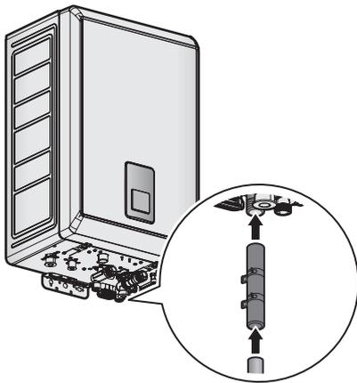
The drain line can be connected to the condensate trap using a condensate trap hose. The hose connection must be secured with a hose clip.
