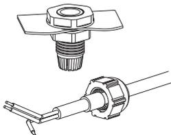
4. Insert all these elements in the cable gland and press on the lid "A" until the cable is sufficiently fixed in place and the unit is sealed.
