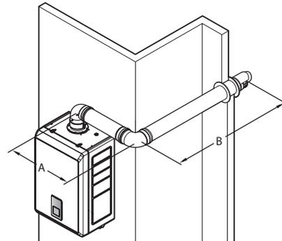
Ø60/100 => Max. length: A+B-(1 x 90°elbow) = 20-2.4=17.6 m
