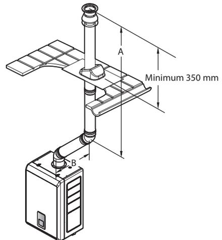
$\text{Ø}60/100 \Rightarrow \text{Max. length: } A+B-(1 \times 45^\circ \text{elbow}) = 21-1.2=19.8 \text{ m}$
