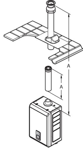
$\text{Ø}60/100 \Rightarrow \text{Max. length: } A=21 \text{ m}$
