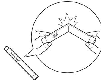
3. When the liquid comes out of the head of the primer stick, apply primer to the back of the bracket and the wall where the NaviCirc is attached.
