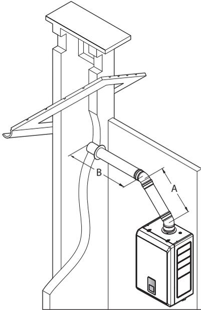
$\text{Ø}60/100 \Rightarrow \text{Max. length: } A+B-(1 \times 45^\circ \text{elbow}) = 20-1.2=18.8 \text{ m}$
