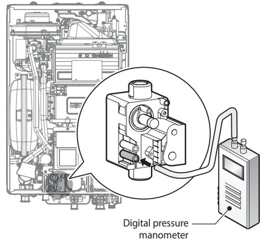
6. Re-open the manual gas valve and check for leaks.
