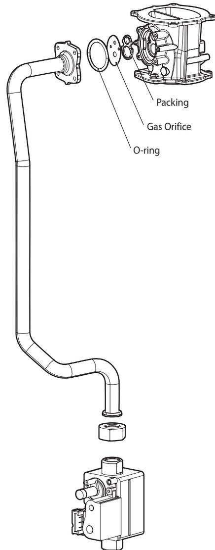
Figure 5-2. Exploded View of Gas Pipe Assembly (NCB700-3S/54K)
