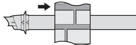
4. Ensure flue weather seal is fitted correctly to ensure a good weathered seal. Then the internal (white) decorative weather seal can be fitted.
