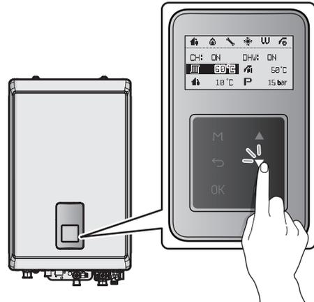
2. Press the OK button (OK) to select the central heating temperature (CH). The highlighted section will flash.
