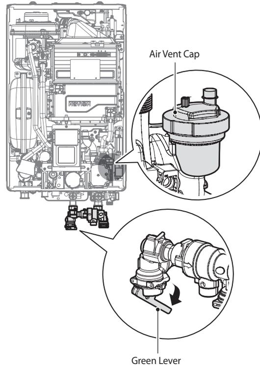
1. Before filling the boiler pipes, unscrew the air vent cap to allow the pipes to fill properly. Screw up the cap when the pipes are full.
