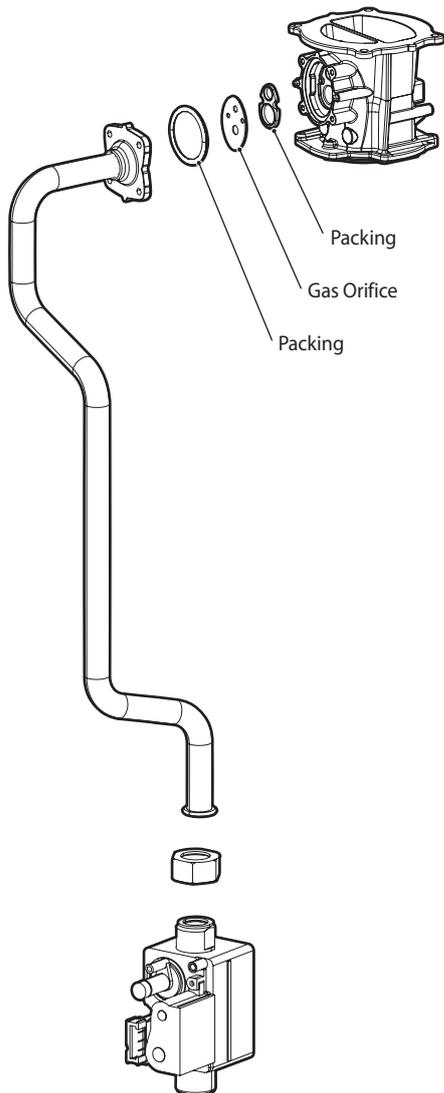
Figure 5-1. Exploded View of Gas Pipe Assembly (NCB700-2S+/42K)
