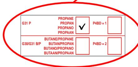
In case of gas conversion, paste the corresponding sticker at the appropriate position in the boiler and mark the square for the used gas type. Because it is not necessary to set parameter P4BD leave the square for parameter B4BD blank.
