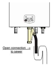
The condensate drain has a 19mm flexible discharge hose. The siphon must always be filled with water. As a safety measure, the siphon has been provided with a floating ball, which closes the outlet in case of water absence, preventing large flue gas leakage.
