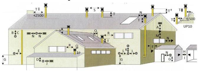
All measurements are in mm are minimum.
