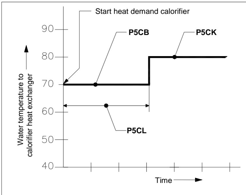
The reason for this function is that the boiler by supplying a lower flow temperature to the heat exchanger of the calorifier, can stay in its condensing mode (if the temperature is low enough) and thus operate at a higher efficiency level. When it takes too long (> **P5 CL**) to heat up the tank with this low temperature mode, the flow temperature set point will change to a higher setting to make sure that the hot water set point is reached.
