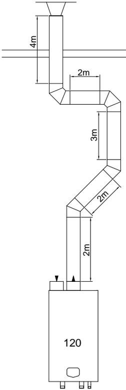
Calculation example with given lengths: checking resistance
