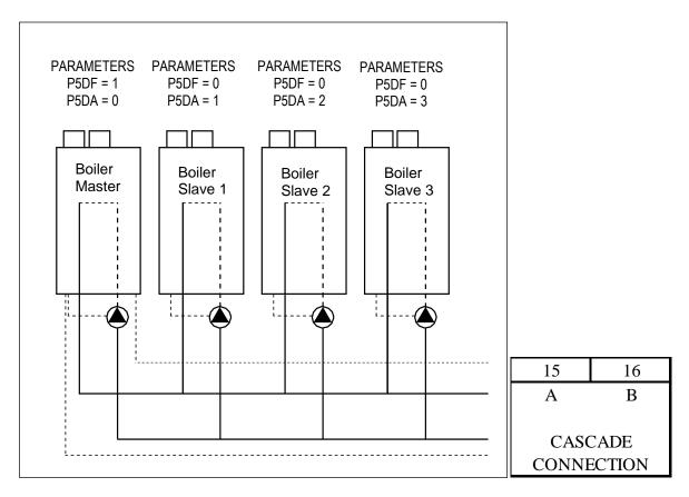
Now for every single boiler of the cascade the following two parameters must be selected and programmed according to the above drawing.
