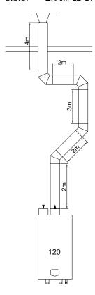
Calculation example with given lengths: checking resistance
