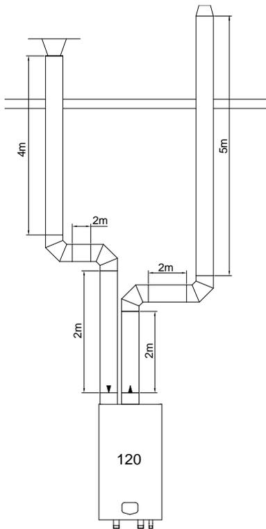
Calculation example with given lengths: checking resistance
