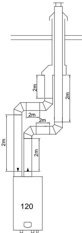
Calculation example with given lengths: checking resistance
