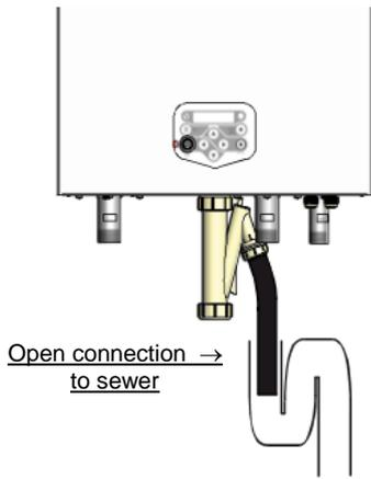
The condensate drain has a 19mm flexible discharge hose. The siphon must always be filled with water. As a safety measure, the siphon has been provided with a floating ball, which closes the outlet in case of water absence, preventing large flue gas leakage.
