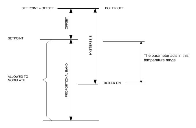
P2KH Gradient heat demand detect DHW tank temperature (display BG)
