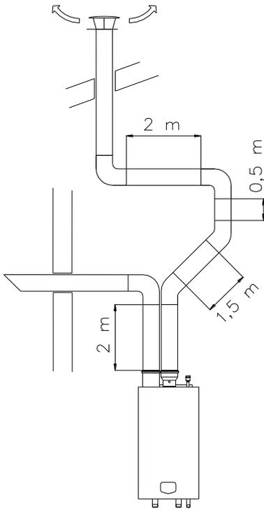
Calculation example with given lengths: checking resistance
