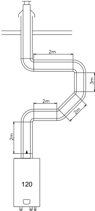
Calculation example with given lengths: checking resistance
