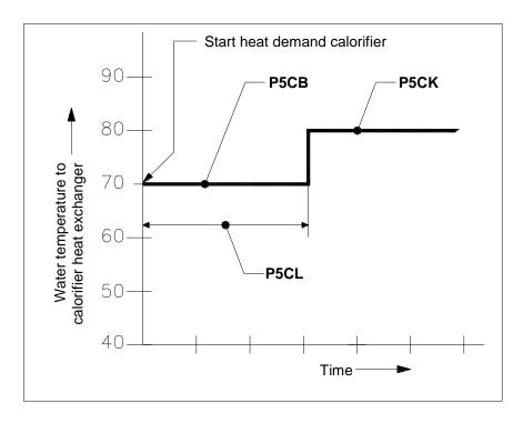
The reason for this function is that the boiler by supplying a lower flow temperature to the heat exchanger of the calorifier, can stay in its condensing mode (if the temperature is low enough) and thus operate at a higher efficiency level. When it takes too long (> **P5 CL**) to heat up the tank with this low temperature mode, the flow temperature set point will change to a higher setting to make sure that the hot water set point is reached.
