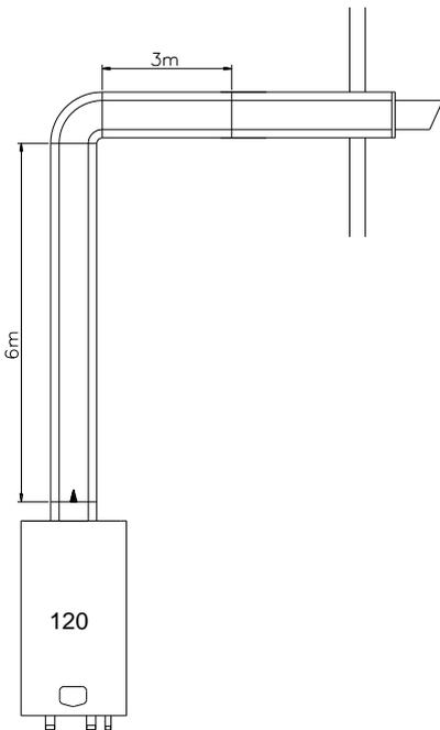
Calculation example with given lengths: checking resistance
