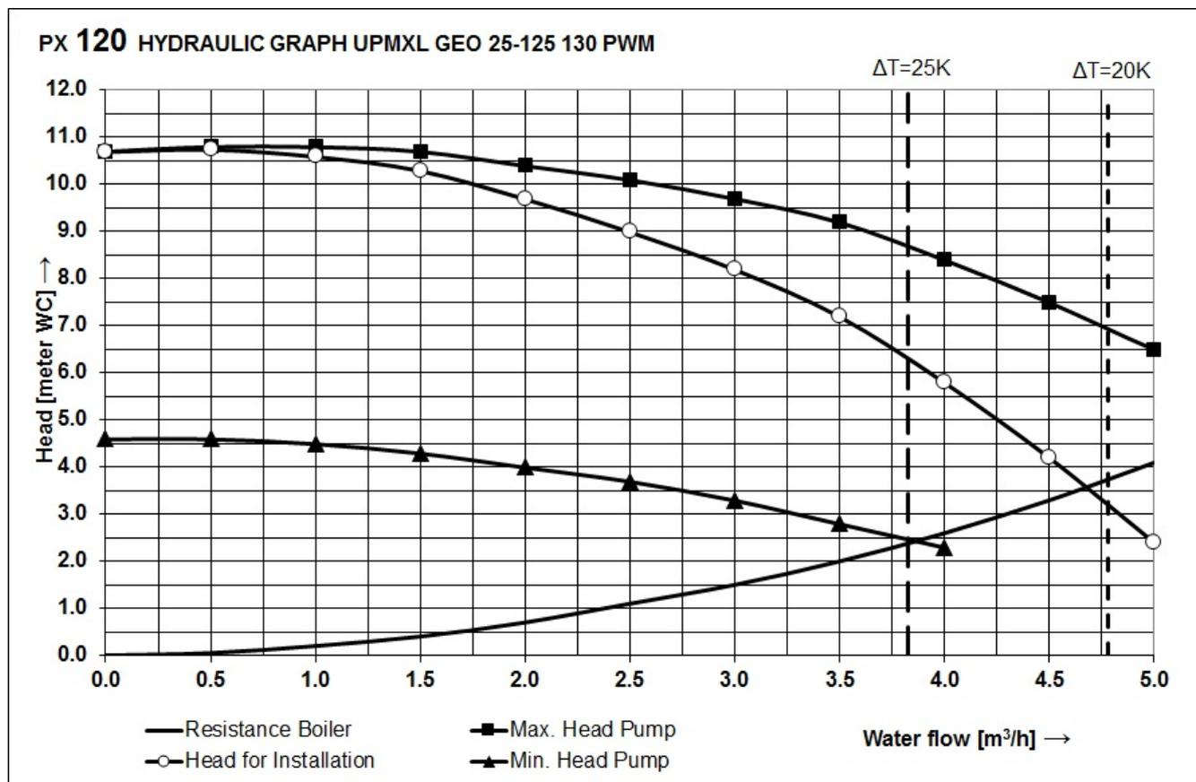
“Head Pump” characteristic line based on the UPMXL 25-125 130 PWM pump.
