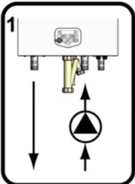
1. Connect the pump hydraulically to the return connection of the boiler and the system
