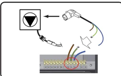
4. Use one of the spare cable glands in the bottom plate to assemble the cable into the boiler.
