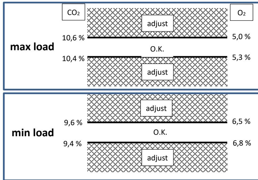
14.1.3. SETTING SCREWS GAS VALVE: DRAWING
