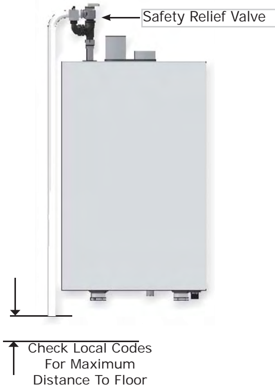
FIGURE 5-2 Safety Relief Valve Discharge Piping
