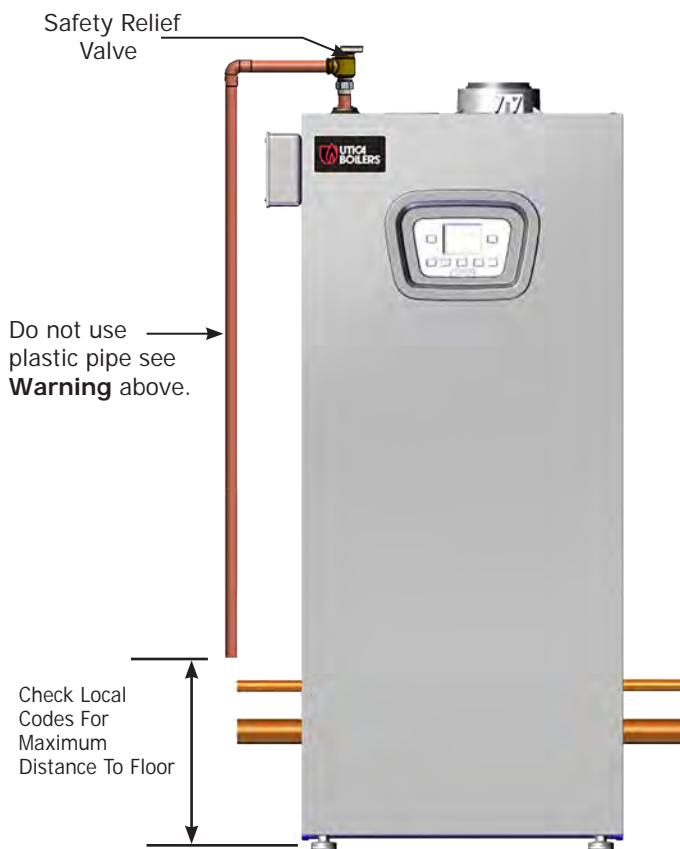
FIGURE 6-1 Safety Relief Valve
