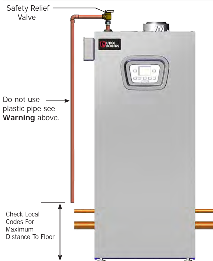
FIGURE 6-1 Safety Relief Valve
