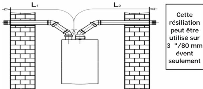
**FIGURE 5-9 – 3 po PIPE DE JUEAU LA RÉSILIATION DE CONDUIT HORIZONTALE SÉPARÉE AVEC LE TEE SUR LA SOUPAPE D’ÉCHAPPEMENT**
