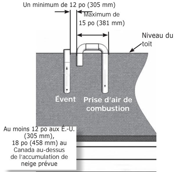
**FIGURE 5-15 – (3 PO/ 80 MM) KIT D'ÉCHAPPEMENT SIMPLE PARI ET DISTANCE MINIMALE D'ENTRÉE D'AIR CENTRE À CENTRE D'UN CENTRE**
