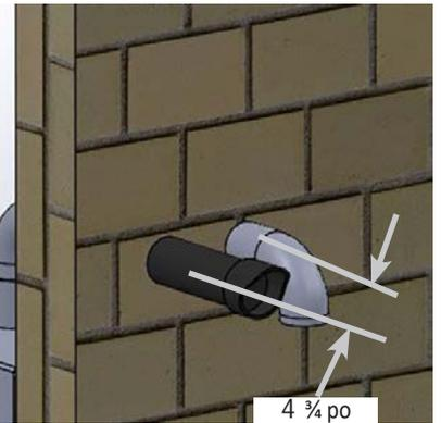
**FIGURE 5-16 – (3 PO/80MM) TUYAU DOUBLE HORIZONTAL, ÉVACUATION ET PRISE D'AIR**
