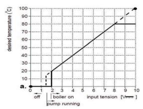
5. Analog Heat Output - Based Control - 0-10V signal controls boiler output between 0% and 100%. Minimum and maximum values are limited. Minimum output is linked to boiler's modulation depth. Output varies between minimum and maximum value on basis of value determined by controller.
