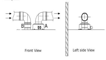
FIGURE 6-6 - Separated Horizontal Flue Termination
