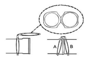
Mechanical fastener is necessary for dual flue pipe.
