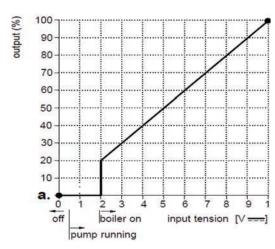
Dependent on minimum modulation depth (set speeds, standard 20%)
