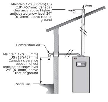
Fig. 6-12 Flue on Sidewall, Combustion Air on Roof
