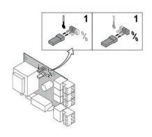
**6.** Analog Output - 0-10V - Temperature or heat output can be chosen for this feedback message. The two controls are described briefly below. Jumper 1 on the interface is used to select either
