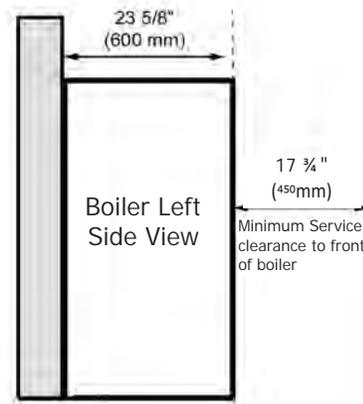
**FIGURE 4-1b Clearance to Combustible Materials**
