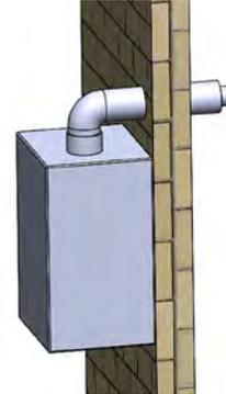
2. **Twin Pipe** – Figure Exhaust and intake air are separate pipes, can be terminated using single wall terminals from the vent manufacturer or field built configuration using elbows or tees.
