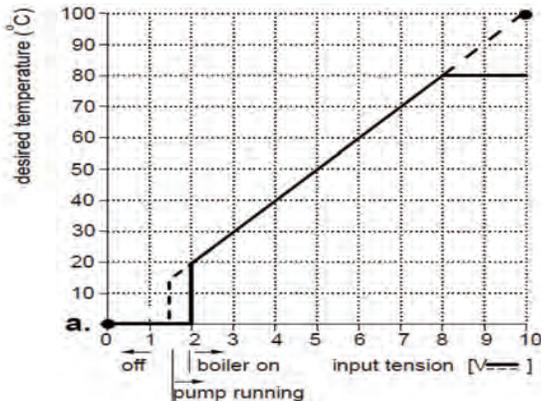
**FIGURE 8-7 Analog Temperature Based Control**
