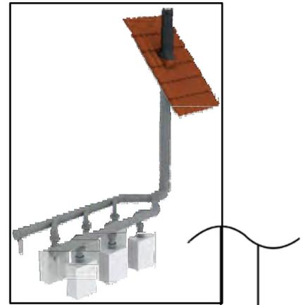
**FIGURE 6-29 - Multiple Boiler Vent Applications**
