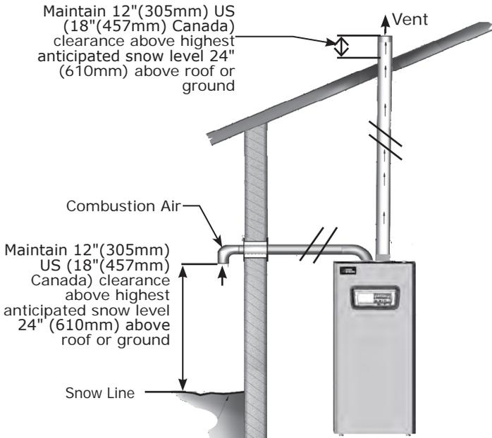
**Fig. 6-12 Flue on Sidewall, Combustion Air on Roof**
