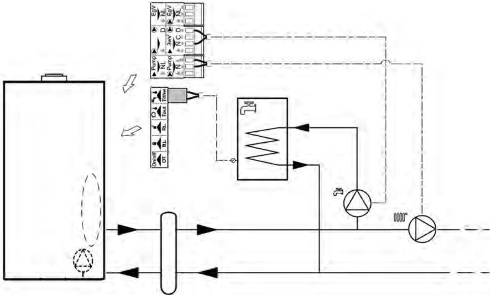
**FIGURE 8-15 Example Of System Shutdown Input Connection**
