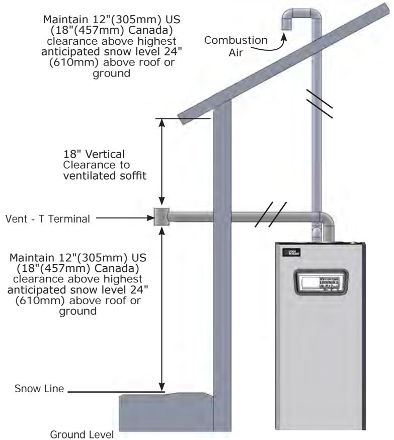
**FIGURE 6-13 Flue on Roof, Indoor Combustion Air**
