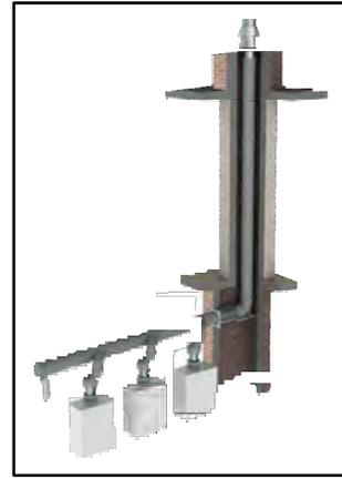
**FIGURE 6-27 - Multiple Boiler Vent Applications**
