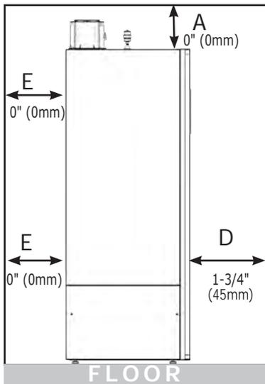
**FIGURE 4-2c Combustible Clearances - Closet Installation**
