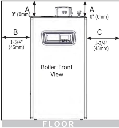
**FIGURE 4-2a Service Clearances - Boiler Front View**
