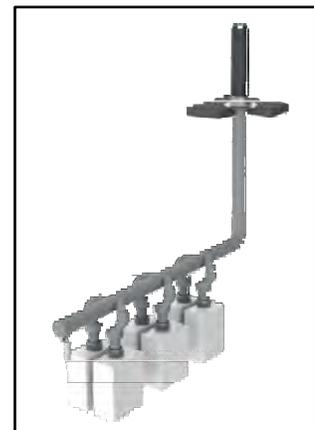
**FIGURE 6-28 - Multiple Boiler Vent Applications**
