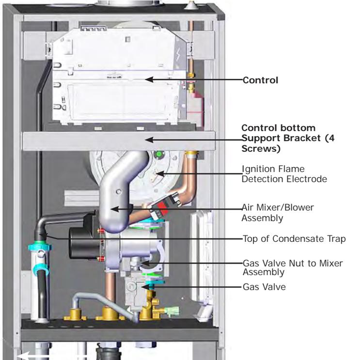
23. Re-install hose to condensate trap. See Figure 5.
