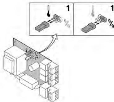
**5. Analog Heat Output - Based Control - 0-10V** signal controls boiler output between 0% and 100%. Minimum and maximum values are limited. Minimum output is linked to boiler's modulation depth. Output varies between minimum and maximum value on basis of value determined by controller.
