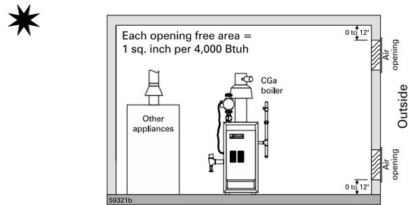
Figure 4 Air from outdoors – vertical ducts
