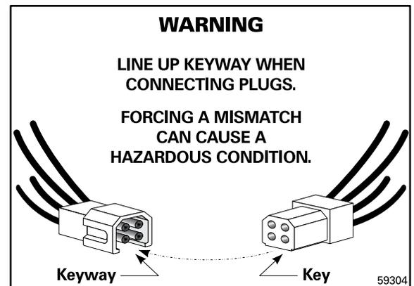
4. Read and apply the harness plug warning label (shown above) so that it is visible after installation.
