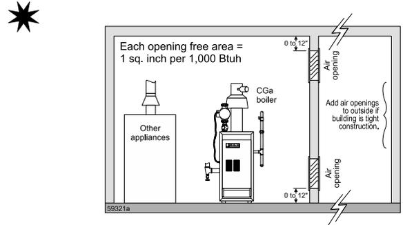
Figure 3 Air directly through outside wall
