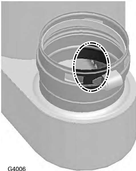
Figure 83 Recuperator flue way drain holes
