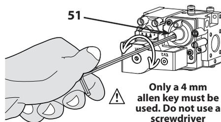
Set the content by turning the screw about a 1/4 of a turn then wait after each change for approximately 1 minute for the CO<sub>2</sub> value to stabilise, then repeat.
