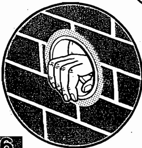
Make good between the edge of the liner and the outside wall with cement mortar or a similar substance, by reaching through the liner and pressing the mortar between liner and the outside brick work. Make good between the liner and the inside wall. Apply soap solution to the 'O' ring inside the liner.
