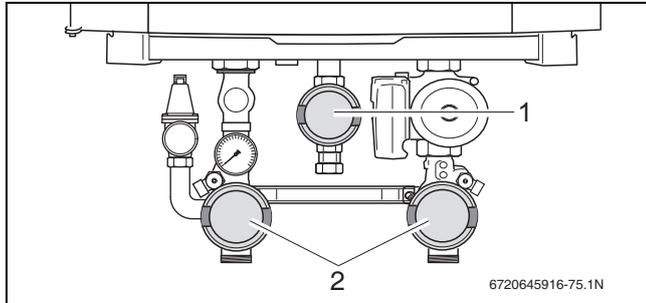
Fig. 77 Closing the valves (here: in closed position)
