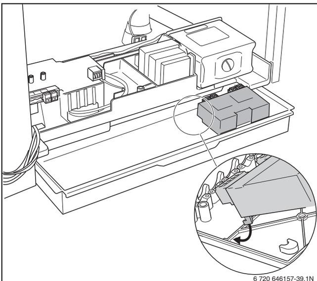
Fig. 43 Clicking the function module into position
