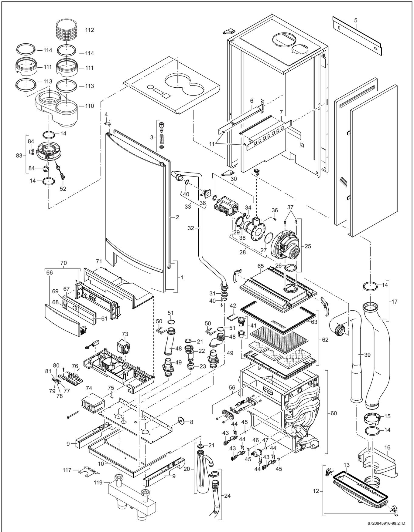
Fig. 101 Exploded view Logamax plus GB162-L.B. 80 kW/100 kW
