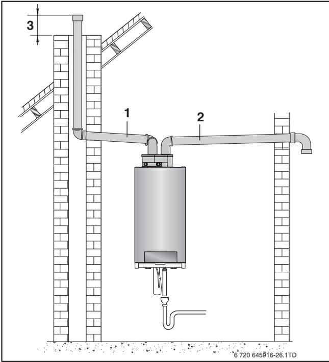
Fig. 30 Vertical venting system (sealed combustion)
