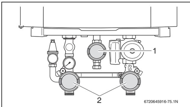
Fig. 80 Closing the valves (here: in closed position)
