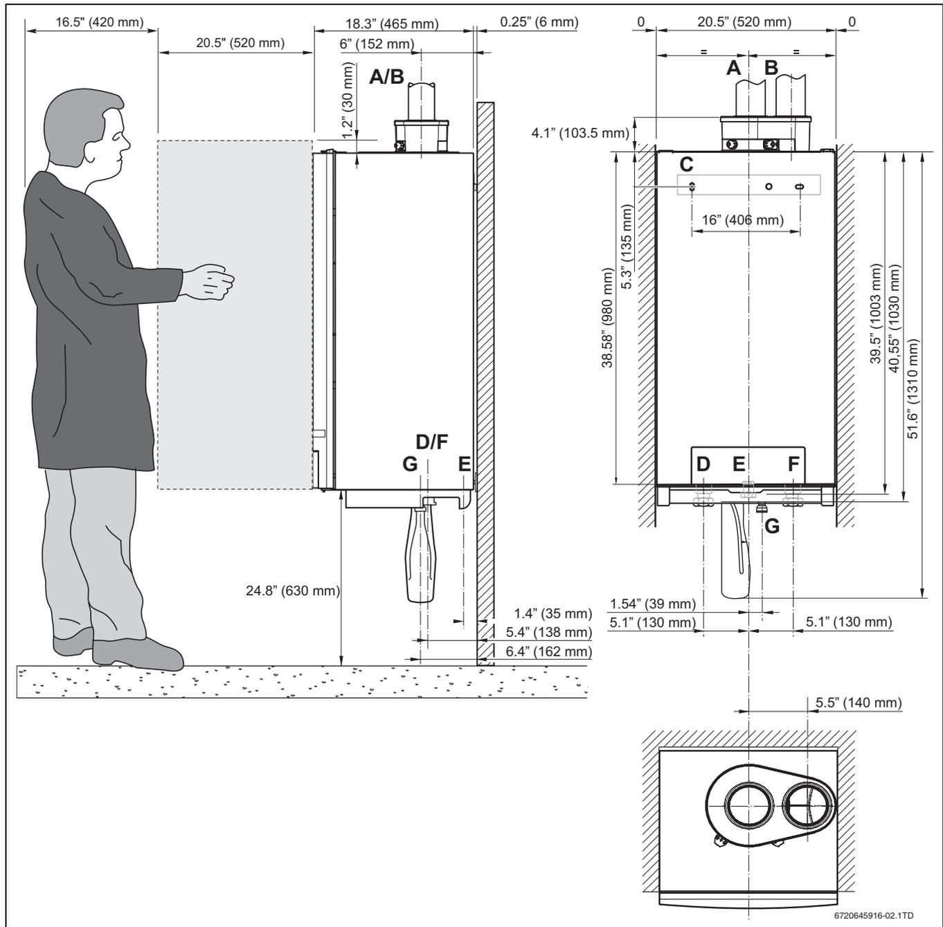
Fig. 2 Dimensions and connections without pump group
