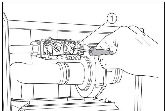
Fig. 69 Adjusting gas/air ratio at minimum load
