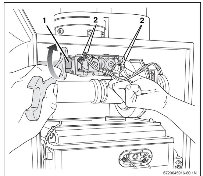
Fig. 82 Undoing the connections to the gas fitting
