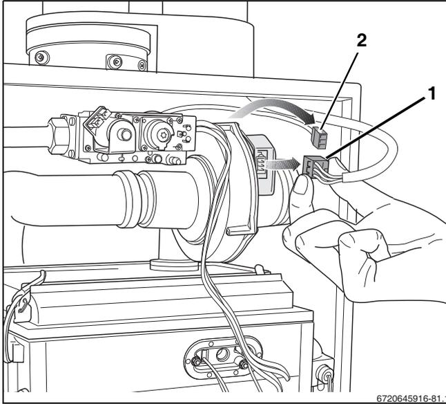
Fig. 83 Removing the connectors from the fan
