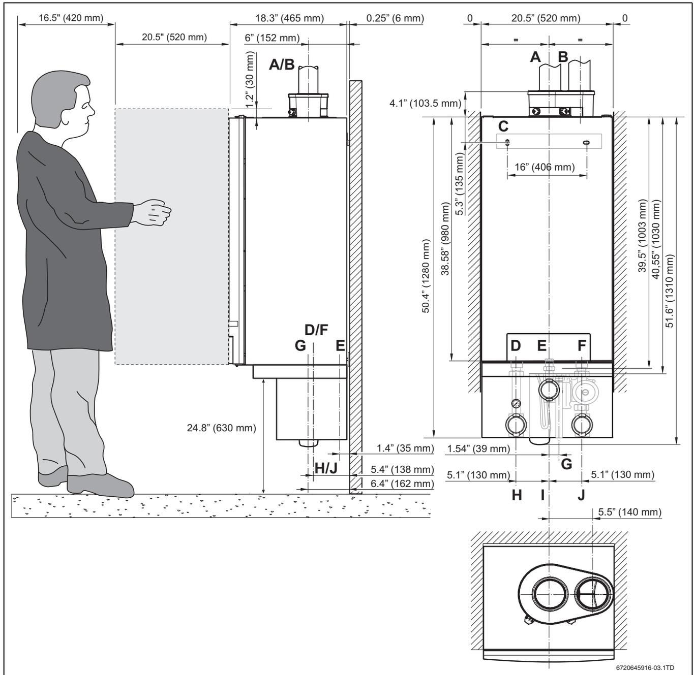
Fig. 3 Dimensions and connections with pump group
