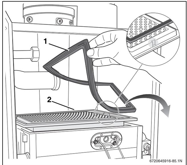
Fig. 87 Removing the burner plate and the burner seal
