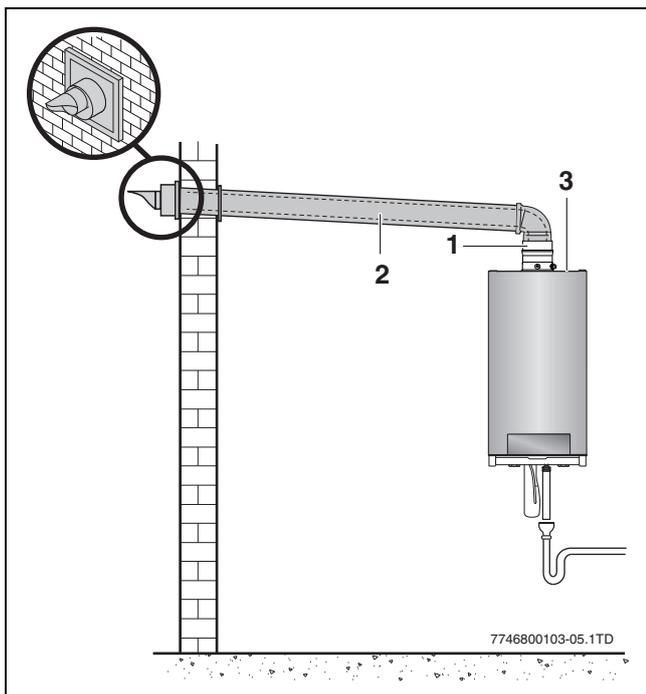
Fig. 27 Concentric horizontal venting system (sealed combustion)
