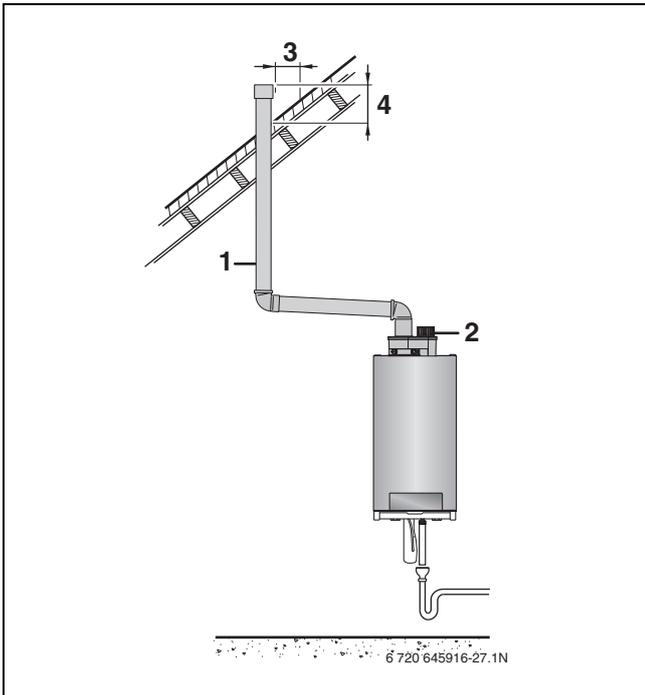
Fig. 31 Vertical venting system (non sealed combustion)
