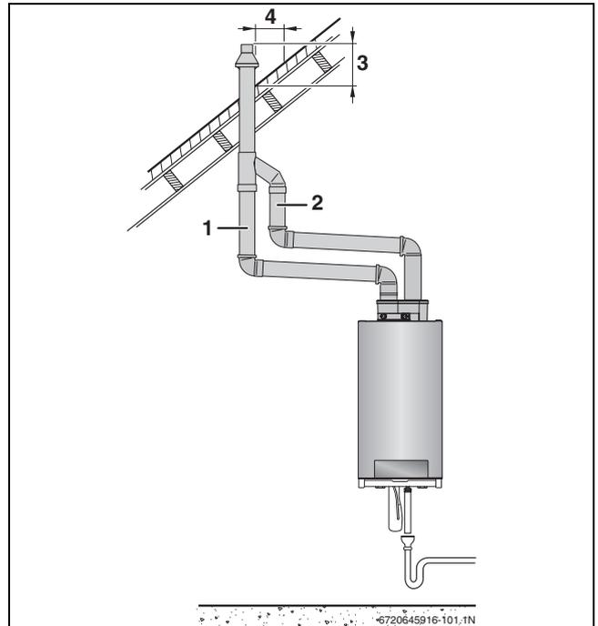
Fig. 33 Vertical concentric venting system (sealed combustion)
