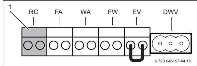
Fig. 48 External connection board - Room controller RC and EMS bus (connection color orange)
