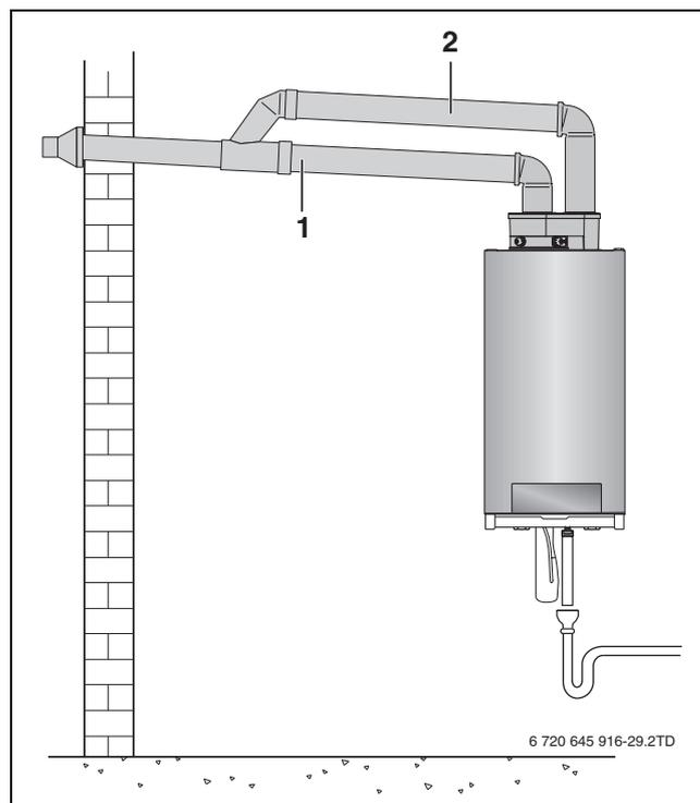
Fig. 28 Horizontal venting system (sealed combustion)
