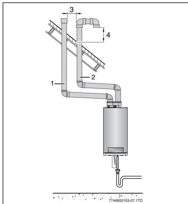
Fig. 29 Vertical parallel venting system (sealed combustion)
