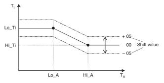
$T_t$  Target water temperature  $T_A$  Ambient (outdoor) temperature Shift value = Shift value
