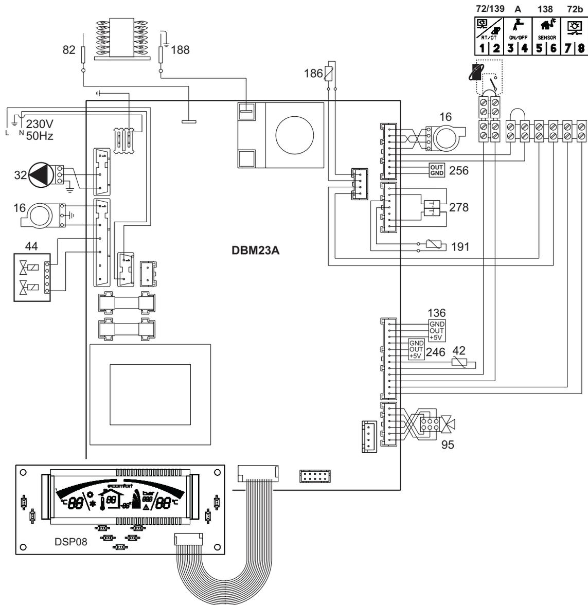
fig. 41 - Wiring diagram
