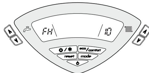
fig. 6 - Boiler lighting
