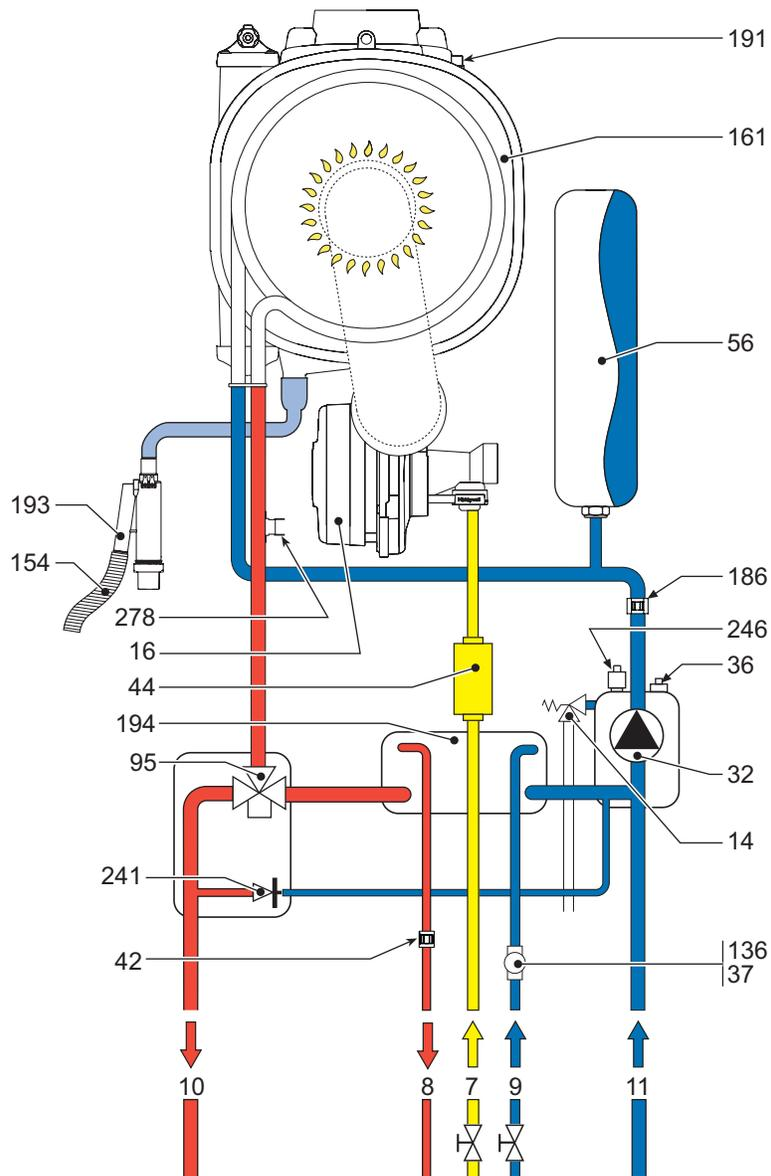
fig. 38 - Water circuit
