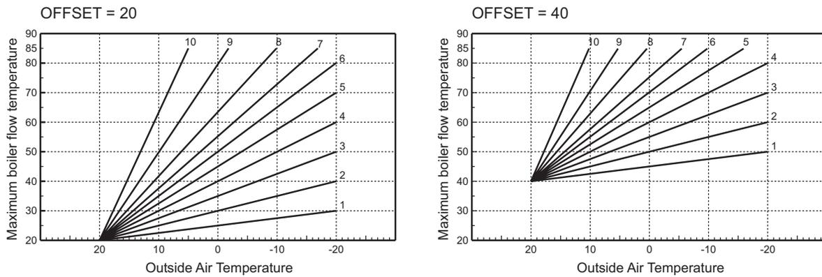
fig. 15 - Example of compensation parallel curve offset
