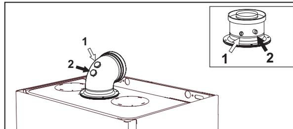
fig. 34 - Flue gas sampling Point
