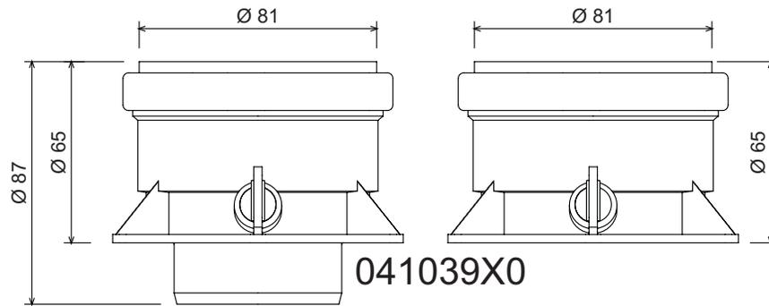
fig. 25 - Starting accessory for separate ducts
