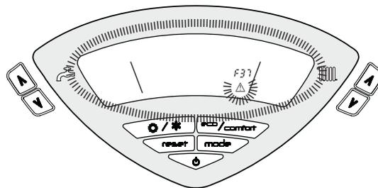
fig. 16 - Low system pressure fault
