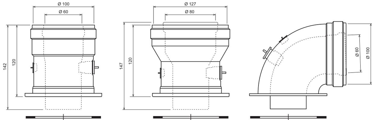
fig. 23 - Starting accessory for coaxial ducts
