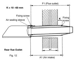
Make sure flue slopes 2° down towards the boiler that is 35 mm fall per metre of flue length
