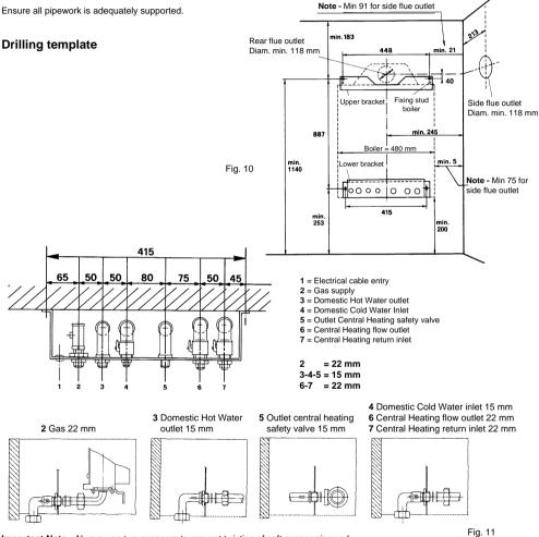
Important Note - Always use two spanners to prevent twisting of soft copper pipework.
