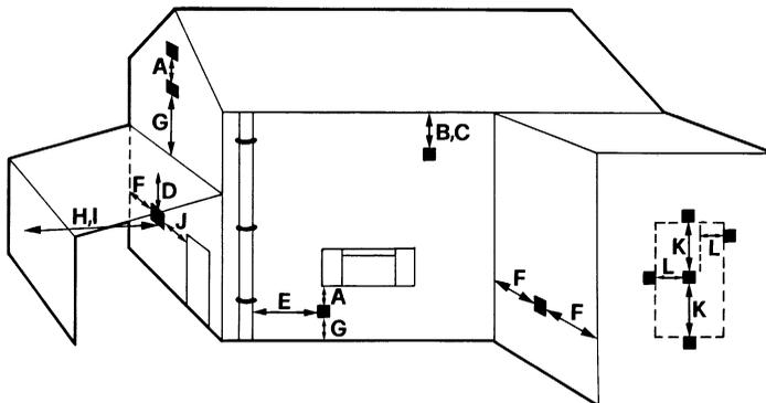
A Quinnell Barratt and Quinnell guard (part. no. C2) should be screwed to the wall centrally over the terminal, when the distance is less than 2 m above a balcony, above ground or above a flat roof to which people have access.
