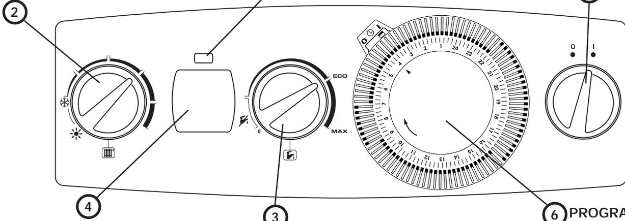
**4 Pressure gauge (bar) and temperature gauge (°C)**
