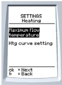
This menu allows you to adjust the installation's maximum heating output temperature (value adjustable between 30 °C and 80 °C - factory setting: 73°C).
