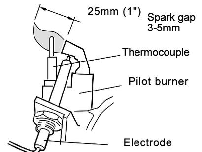
The pilot is factory set to maximum and no further adjustment should be necessary. However, if the pilot flame appears small, check the pilot injector. Refer to Frame 39.
