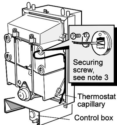
5. Remove the control box fixing screw and pull the box forward and downward to disengage.
