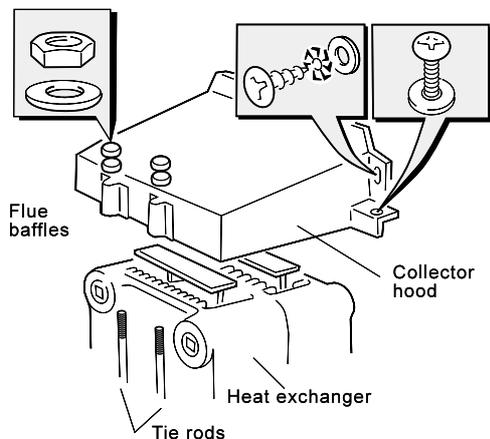
3. Unclip and remove the flue baffles from the heat exchanger.
