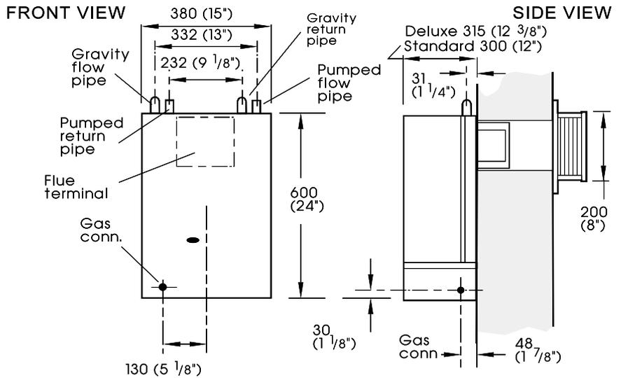
Front clearance; 450mm (17 3/4") from the front of the boiler casing. Minimum front clearance when built in to cupboard is 75mm (3")
