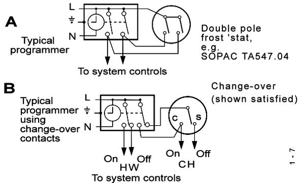
Central heating systems fitted wholly inside the house do not normally require frost protection as the house acts as a 'storage heater' and can normally be left at least 24 hrs. without frost damage. However, if parts of the pipework run outside the house or if the boiler will be left off for more than a day or so, then a frost 'stat' should be wired into the system.
