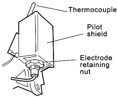
If required, the pilot injector may now be unscrewed and the injector checked or replaced as necessary.
