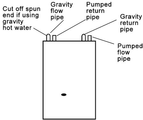
1. This appliance is NOT suitable for use in a direct hot water system.
