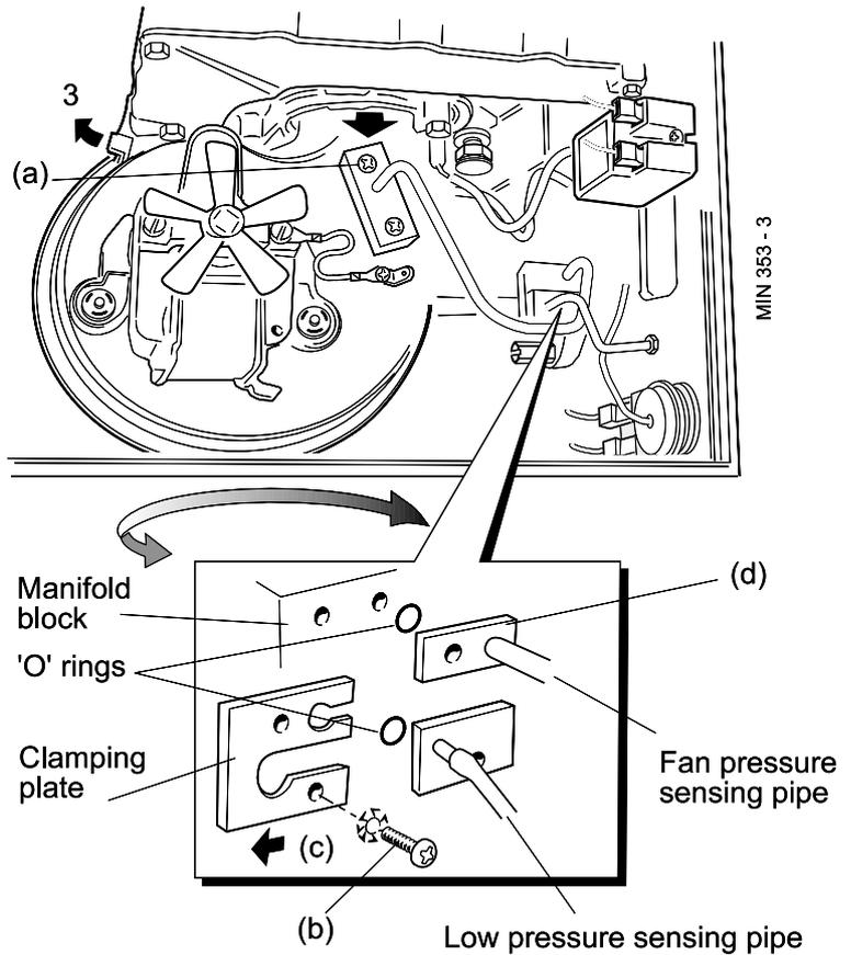
4. Press the retaining bracket lever upward and rotate the fan body to the right to disengage the fan scroll from the bracket. Continue rotating to disengage the bayonet fixing on the fan outlet.
