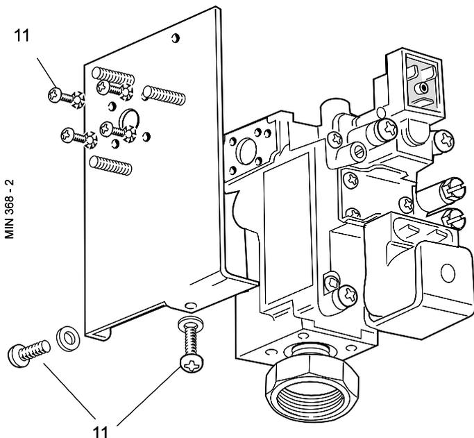
14. Fit the new gas valve in reverse order, ensuring that the gas injection pipe O ring seal is refitted.
