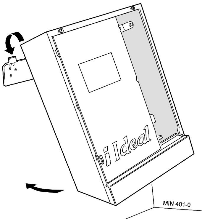
1. Lift the boiler onto the wall mounting plate, as shown.
