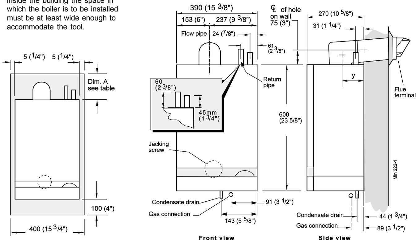
Front clearance: 450mm (17 3/4") from the front of the boiler casing.
