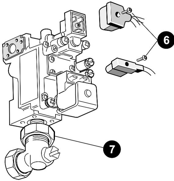
6. Undo the 2 retaining screws and unplug the electrical leads from the gas valve.
