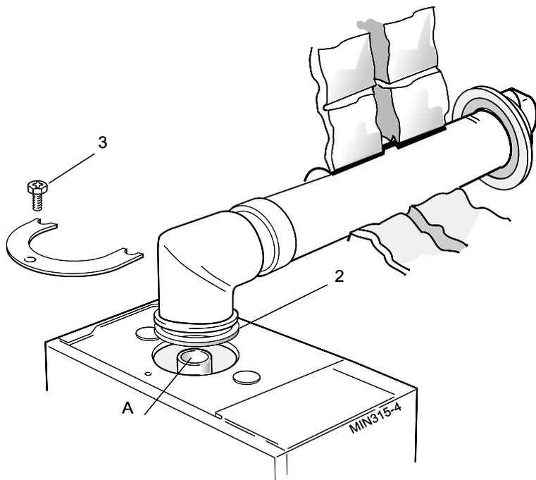
**Note.** BEFORE fitting the flue turret, fill the condensate siphon within the boiler by pouring a cupful of water into the flue outlet A.
