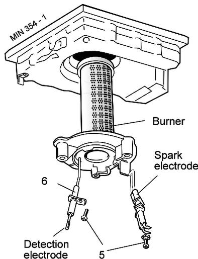
9. Check the ignition and operation of the burner.
