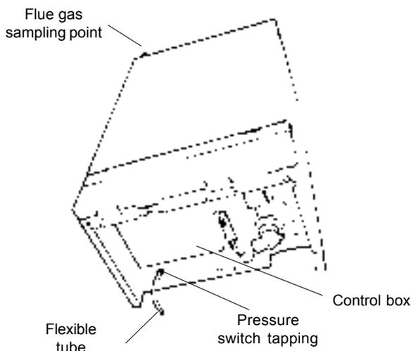
3. With the boiler running, blow gently into the tube. The burner should shut down and the 'Burner on' neon extinguish. The fan should continue to run. If this does not occur replace the pressure switch - refer to Frame 71.
