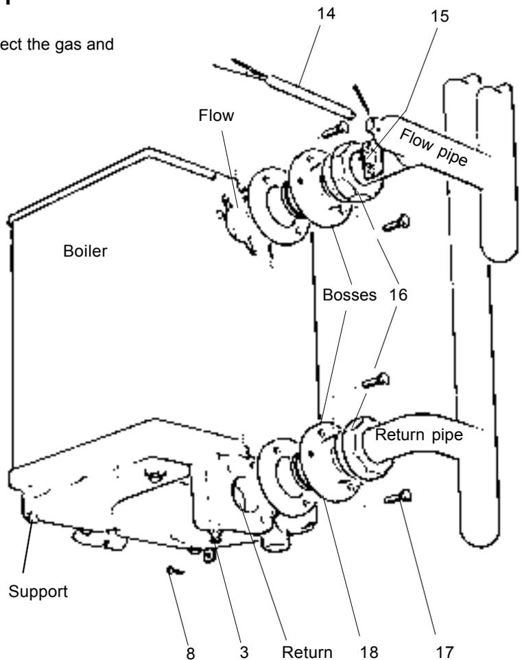
13. Disconnect the boiler flow and return pipes from the system pipework close to the boiler.
