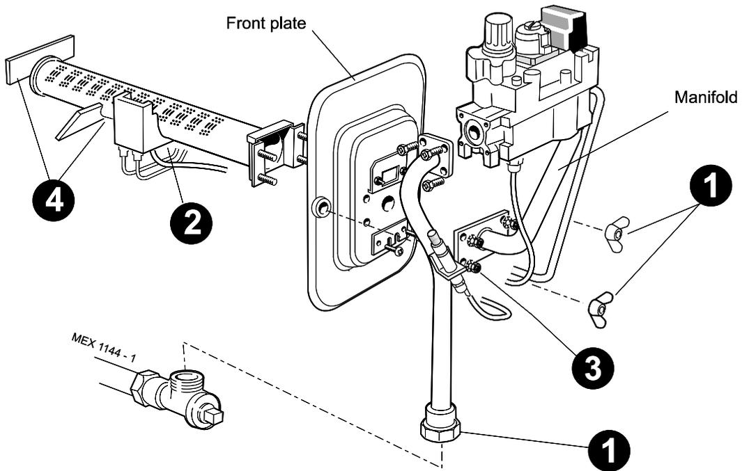
1. Lift off lower front panel and remove the grille assembly. Refer to Frames 28 & 29. Undo the gas cock union and the 2 wing nuts to remove the burner and controls assembly.
