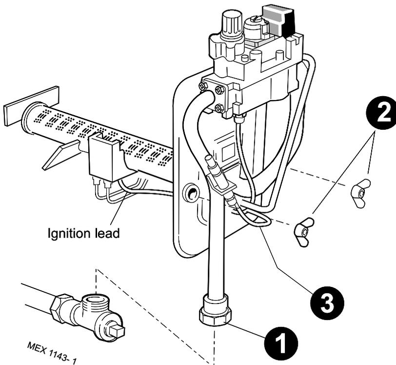
1. Lift off lower front panel and remove the grille assembly. Refer to Frames 28 & 29. Undo the gas cock union.
