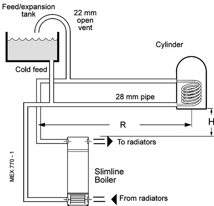
**R** = the horizontal distance between the centre line of the cylinder and the boiler tapplings used (measured along the pipe run).
