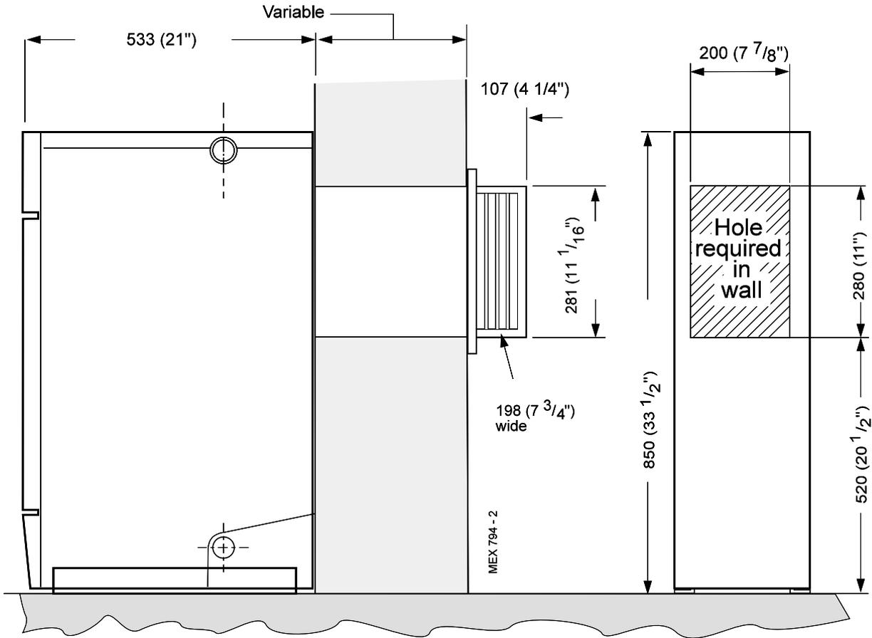
1. Cut the appropriate hole in the wall for insertion of the terminal assembly.
