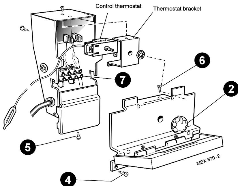
1. Lift off the lower front panel. Refer Frames 28 & 29.
