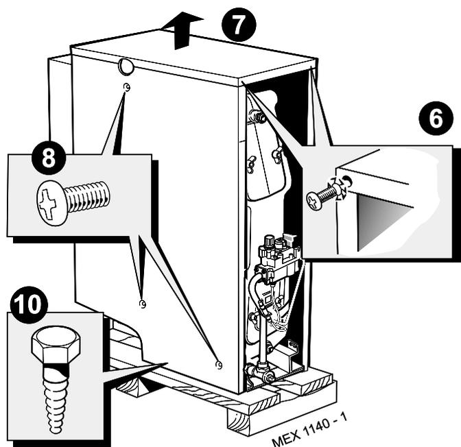
7. Lift the top panel off the boiler.
