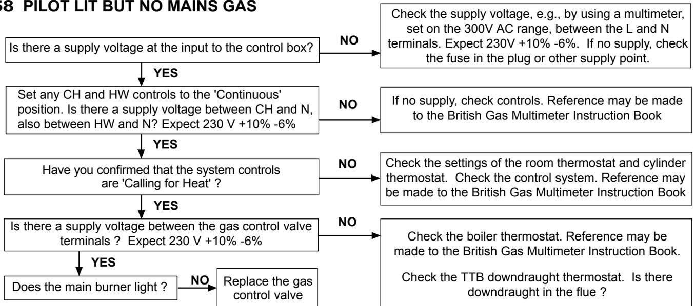
**Note.** After any faults have been corrected, return all thermostatic and other controls to the previously noted settings
