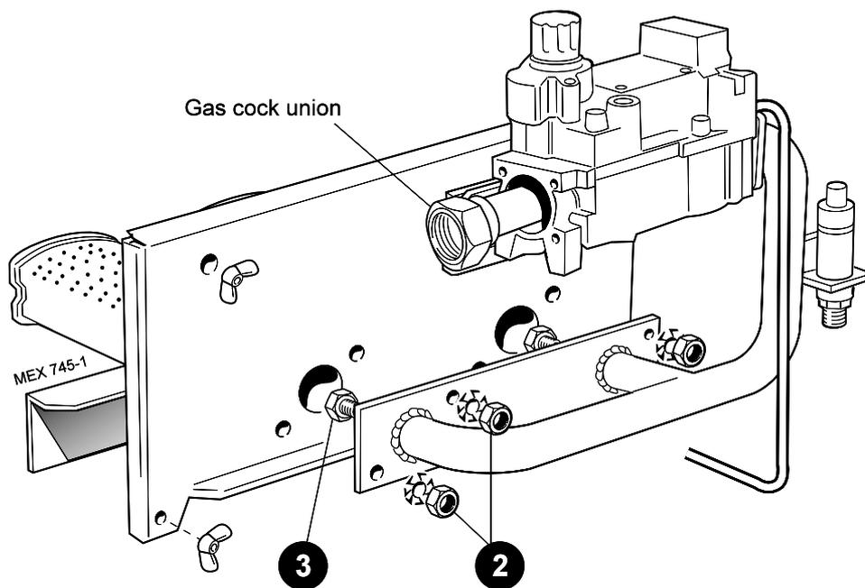
1. Lift off front panel and remove the grille assembly - refer to Frames 28 & 29. Undo the gas cock union. Undo the 4 wing nuts and remove the burner / controls from the boiler.
