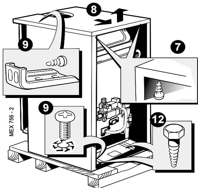
6. Remove the 2 screws securing the top panel to the side.
