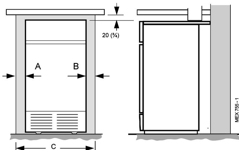
**Note. 3/100P ONLY.** If minimum LH side clearance is used, the TTB downdraught thermostat and bracket should be moved to the RH side of the boiler (alternative location).
