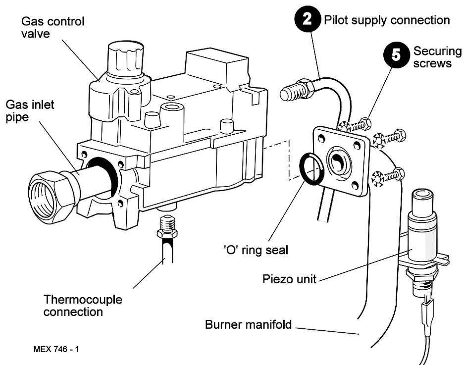
6. Fit the new gas valve, ensuring that:
