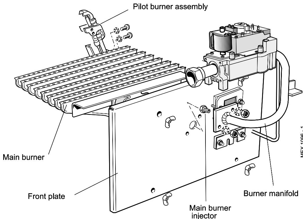
1. Remove the 2 screws and lift off the lower front panel then remove the grille assembly. Refer to Frame 57. Undo the gas cock union. Remove the 4 wing nuts and withdraw the burner and controls assembly, complete, from the boiler.
