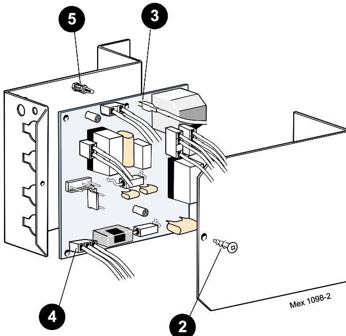
1. Remove the 2 screws and lift off the lower front panel - refer to Frame 57.
