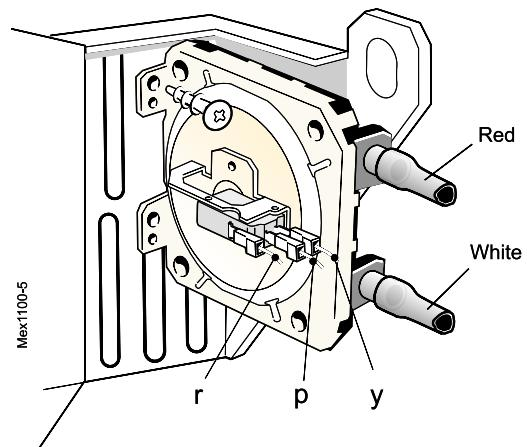
**75 PRINTED CIRCUIT BOARD (PCB) REPLACEMENT**
