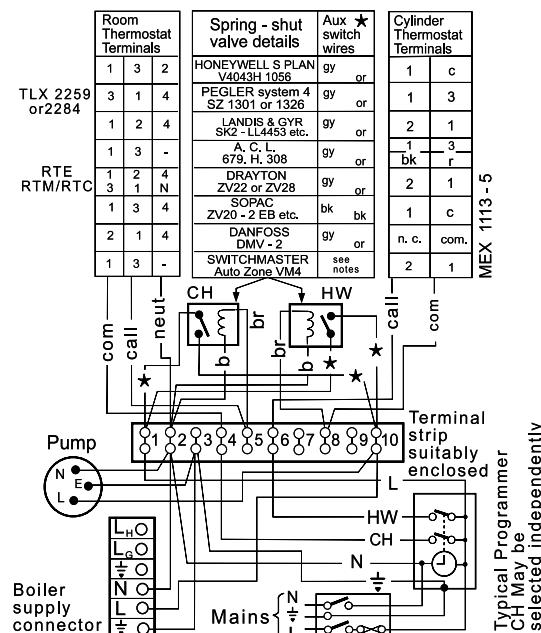
**49 HONEYWELL 'C' PLAN** Gravity HW & Pumped CH
