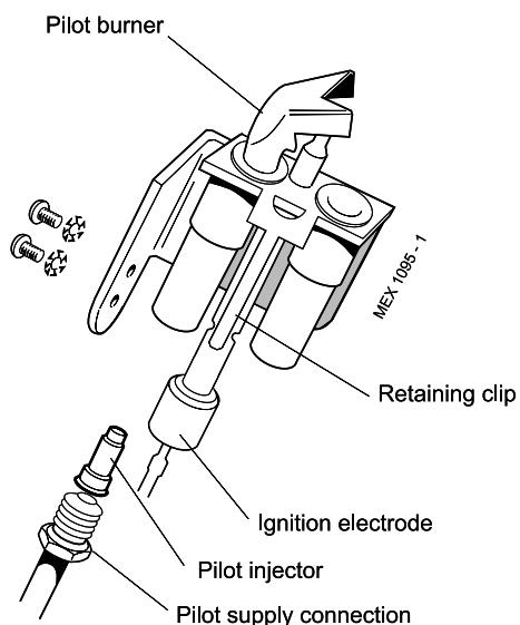
4. Push in the new electrode until the retaining clip locates in the groove and re-assemble in reverse order.
